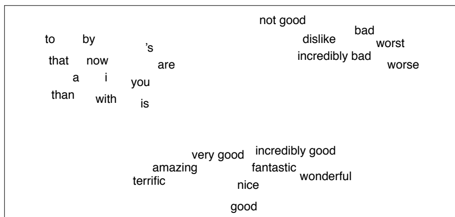
Figure 6.1 A two-dimensional (t-SNE) projection of embeddings for some words and phrases, showing that words with similar meanings are nearby in space. The original 60-dimensional embeddings were trained for sentiment analysis. Simplified from Li et al. (2015).
